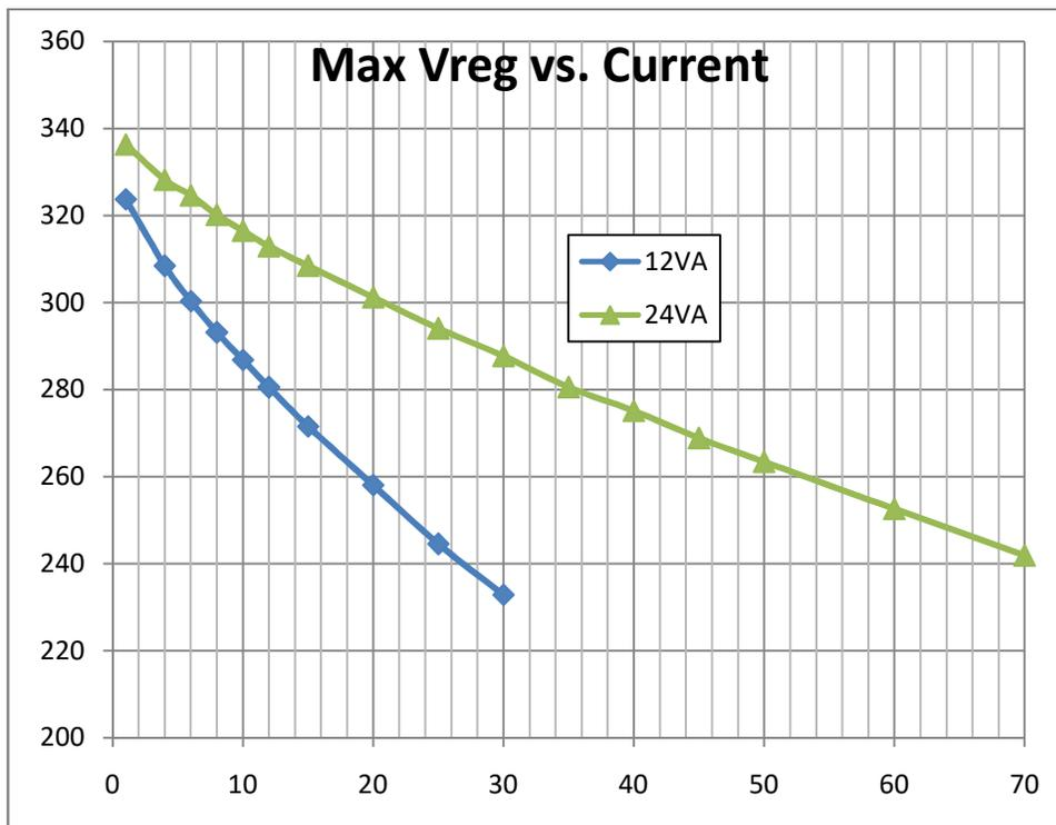
The minimum voltage setting is about 200V with the values in the parts list; current should be limited at lower voltage settings to stay within the regulator's rating. Dissipation in a regulator is  $(V_{in} - V_{out}) \cdot I_{out}$  – should be kept below 4 watts. If an infrared thermometer is available, check that device case temperature doesn't exceed 100 deg C.
