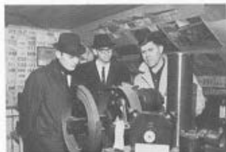
Firing up W2QB's 1000 watt sync rotary spark transmitter always makes a good show if only for a couple "sparks"...
