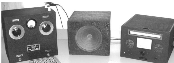
Author's National FB7/Utah Jr. station. Key and receiver power supply not shown.
