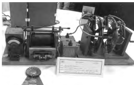
Severin Dvorsky won first in "Spark Transmitters and Receivers" with this home built spark transmitter.
