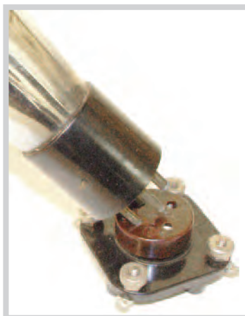
After 1930, tube bases lost side pin, could no longer be bayonet mounted. “Push-in” installation became the standard.
