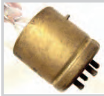
“UV” base had locating/locking pin for bayonet mounting, short contact pins.
