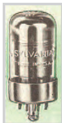
The Loktal tube, originated by Sylvania, had a unique locking groove on its locating pin.
