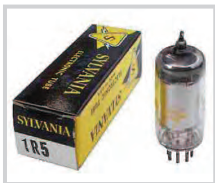
The original miniature tubes, designed for use in battery portables, had 1.4-volt filaments. This is the 1R5 pentagrid converter.
