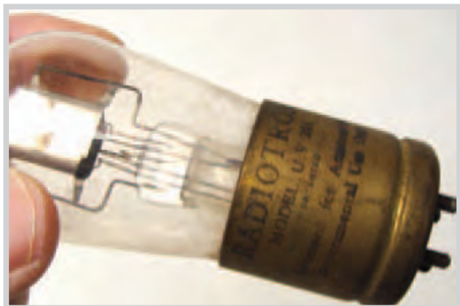
One of the first receiving tubes to reach consumers in quantity was the UV-201.
