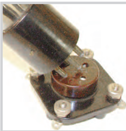
Long contact pins on the UX base slid into matching holes in the tube socket.
