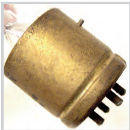
A horizontal locating/locking pin and stubby contact pins are features of the UV-type base.
